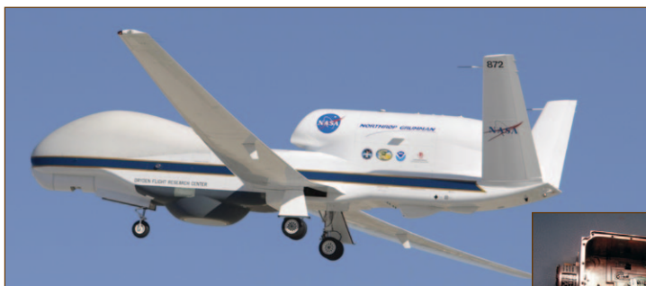
NASA's Global Hawk carrying a synthetic aperture radar payload (inset) on a fully unmanned aerial recon mission uses internal DSP-1750 gyros from KVH to maintain focused and stable imagery.
