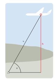
With an extended inclination range of -30° to +90° VECTOR 21 AERO allows measurements such as aircraft position and height above ground, cloud height, flight path of large migratory birds, etc.
